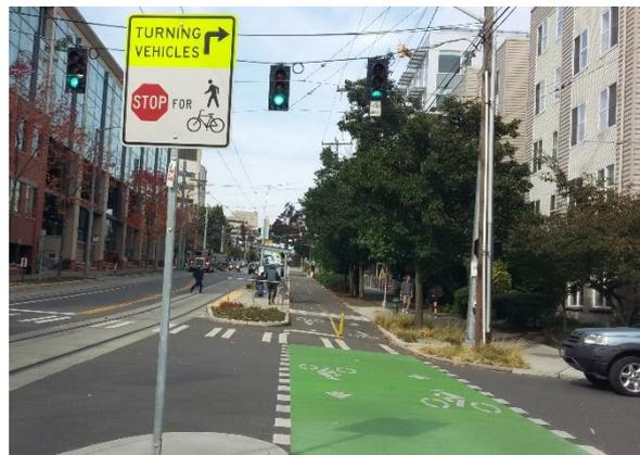
Figure 3: One variation of sign used for filter turning in USA, Broadway, Seattle
