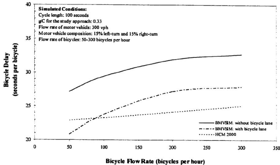
**Figure 2-1: Bicycle delay against bicycle flow rate (Raksuntorn 2002)**
