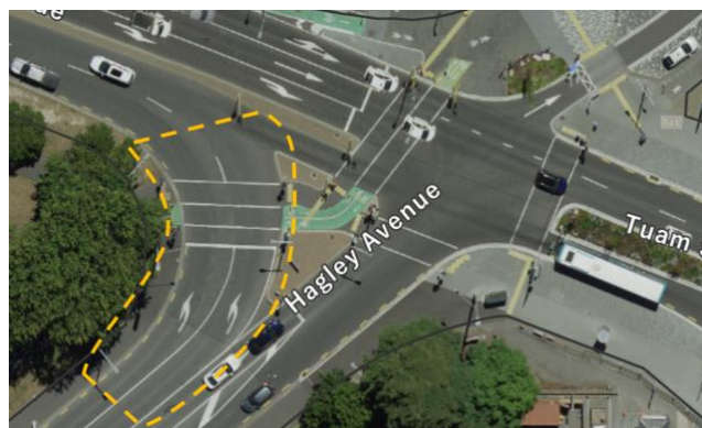
Figure 2-2: Signalised two-lane slip lane (source: Canterbury Maps)
