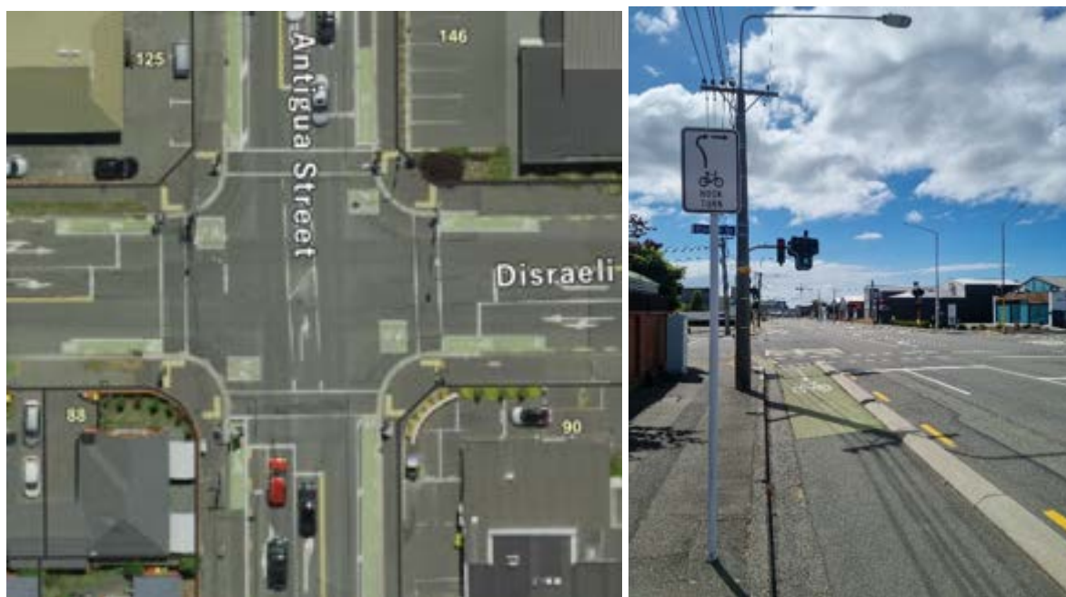
Figure 32-1: Separated cycleway (north-south corridor) with fully protected phasing, Christchurch 7
