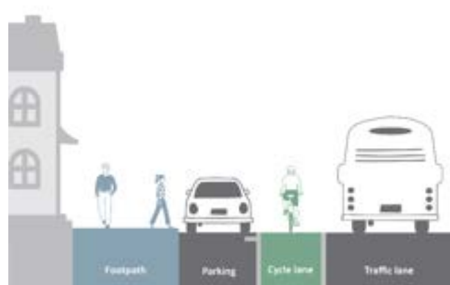
Figure 23-3: Cycle lane next to parking
