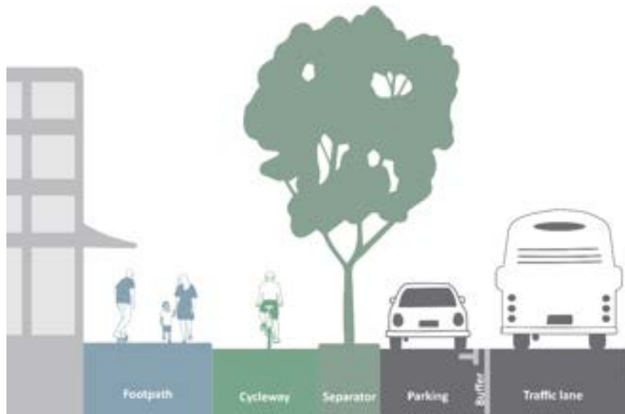
Figure 19-3: Separated one-way cycleway
