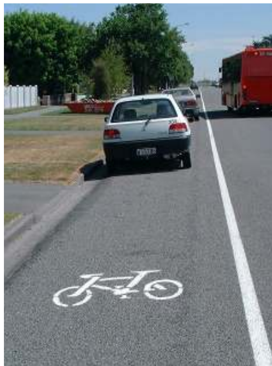
Figure 8: Transit had cycle logos added to the parking lane to make the SH more 'cycle-friendly'
