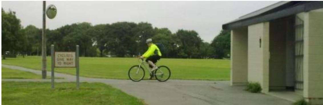
Figure 41: Poor path intersection intervisibility somewhat mitigated by mirror and sign – Hagley Park, Christchurch
