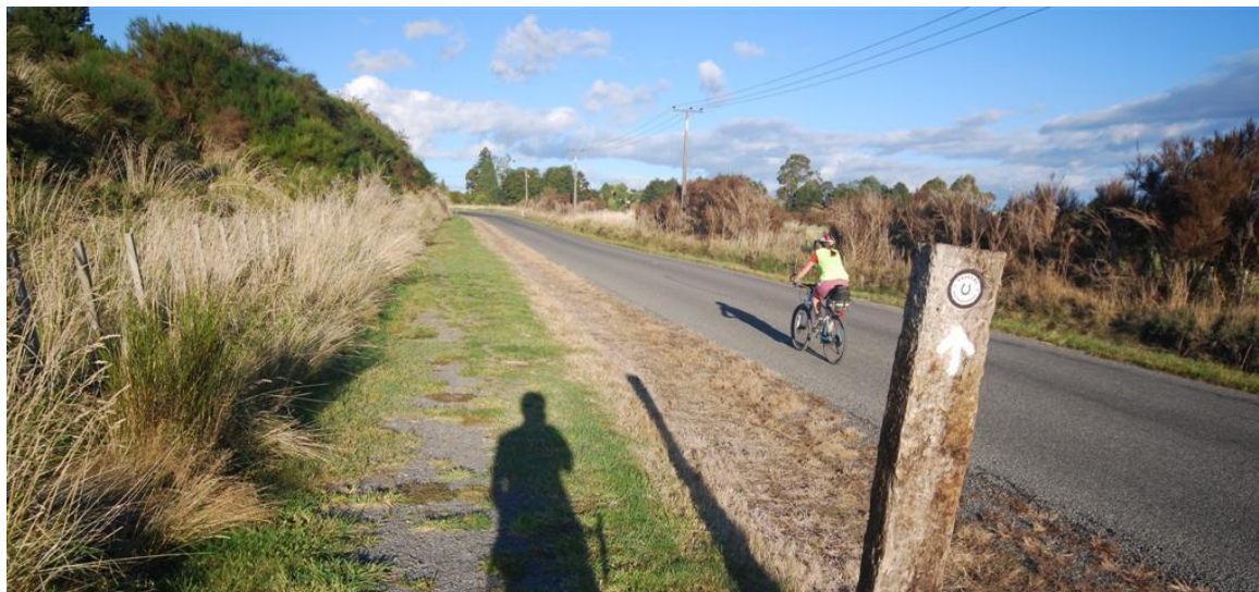
Figure 9: Poorly-surfaced cycle path next to low-volume road will be shunned by cyclists
