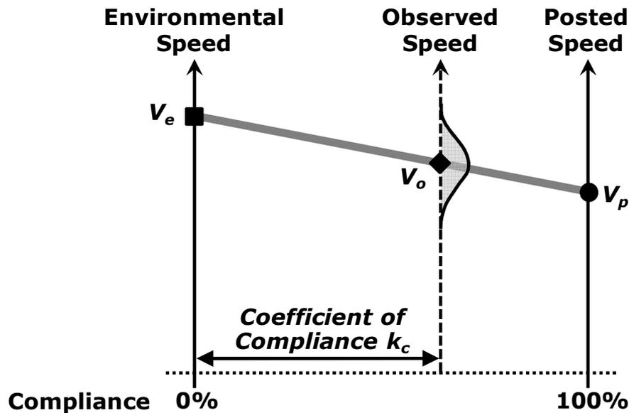
Figure 2: Relationship between Environmental, Posted and Observed Speeds
