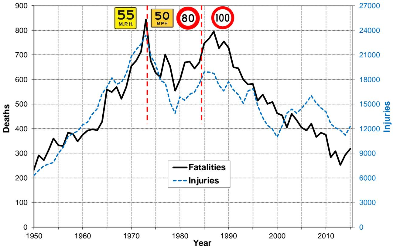
Figure 1: Time series of road deaths and injuries in New Zealand (adapted from MOT 2016)
