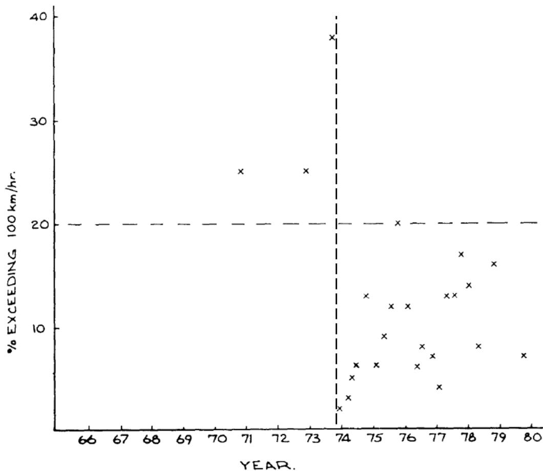
Figure 5: Time series of observed vehicles on rural roads exceeding 100 km/h (Frith & Toomath 1982)
